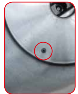
Probe in direct contact with the mix
