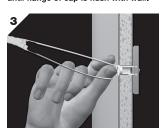
Snap straps at wall by pushing side to side, snapping off straps level with flange of cap.
