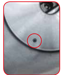
Probe in direct contact with the mix
