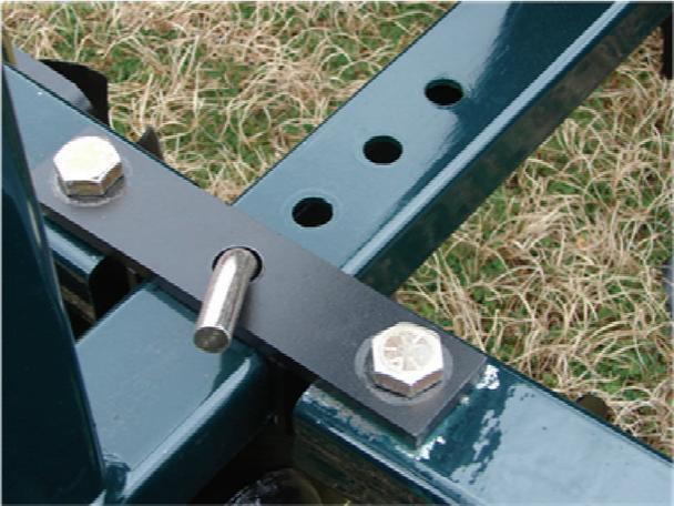
(Above) The Front Gang Assembly has (4) positions that the Gang Assembly can be adjusted. The Front Pin Hole (Shown Above) is the least aggressive and each pin hole moving back will put the gang assembly into more aggressive positions.
