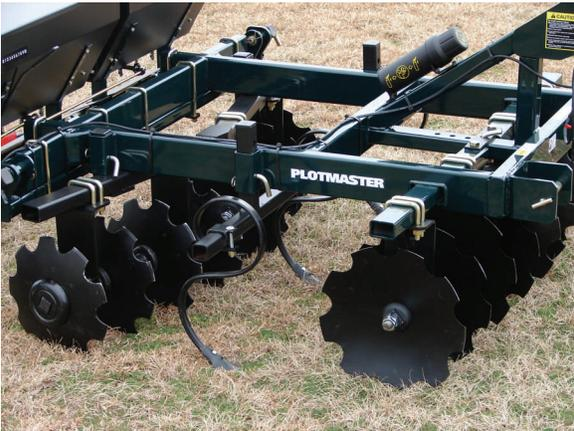
(Above) Side view of unit showing the front gang assembly set to throw tilled dirt outward and the rear gang assembly set for additional tillage and for pulling the tilled dirt from the front gang assembly inward, thus creating an optimal seed bed.
