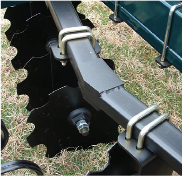
(Above) The Rear "V" Shaped Gang Assembly has a fixed position and is set at a pre-determined angle for maximum tillage. The rear disk can also be used to place soil on top of seed. Depending on travel speed and top link adjustment the soil disturbance can help the dirt flow on top of the seed.
