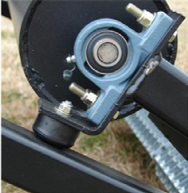
(Above) Hard Rubber Stop for Cultipacker Roller to rest on Drag Arm when not in use. Grease Zerk on Pillow block bearing needs to be filled periodically
