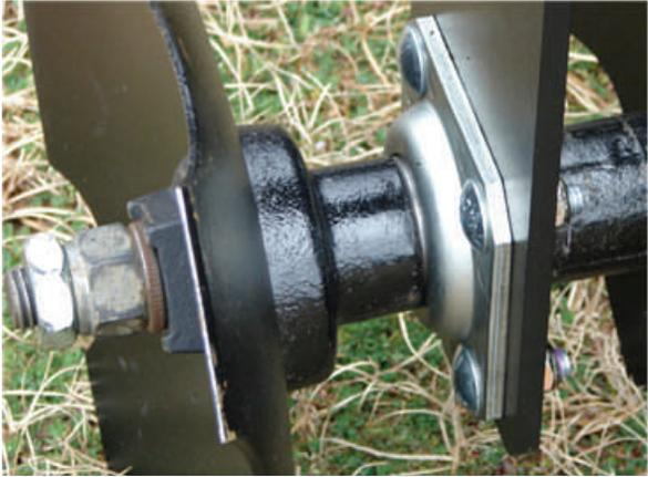
(Above) Non-Greasable Sealed Bearings are used on both front and rear gang assemblies. These increase longer life and dependable use of your unit for years to come.
