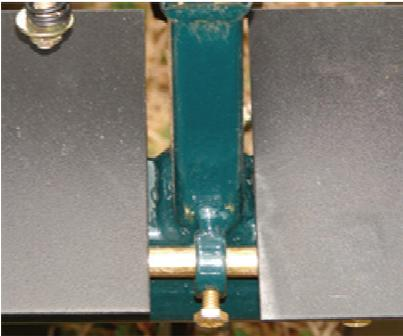
Adjusting Bolt located on Seeder "Y"
