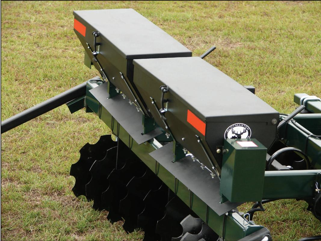
EACH “SPLATTER PLATE” IS DESIGNED TO ALLOW SEED TO SCATTER AND SPREAD EVENLY.
