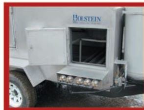
Door to pilot light, burners and gas valve
