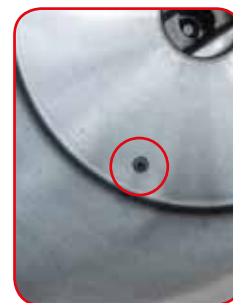
Probe in direct contact with the mix
