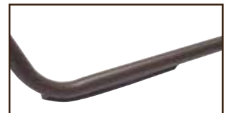
Aluminum skid welded into place
